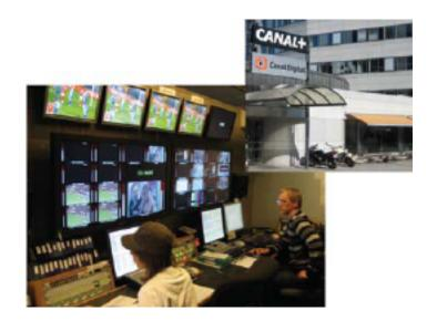
ServSwitch Octet switches were set up to connect the servers to a wall of monitors and to multiple technician KVM stations in the studio. With just a click or two, the technicians can control subtitling, transmission, recording, and broadcasts.
